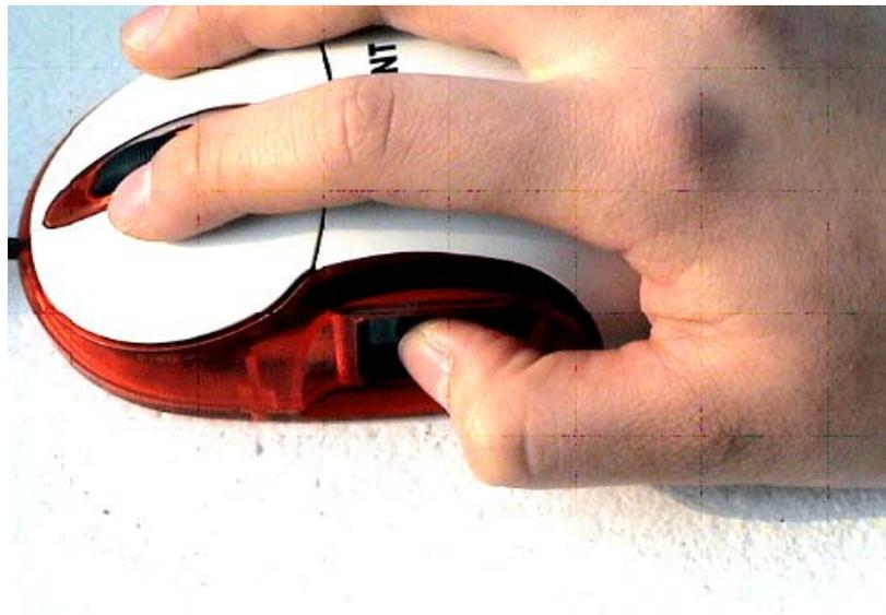
Another WRONG example of finger positioning. The core is slightly to the left of the image sensor.
