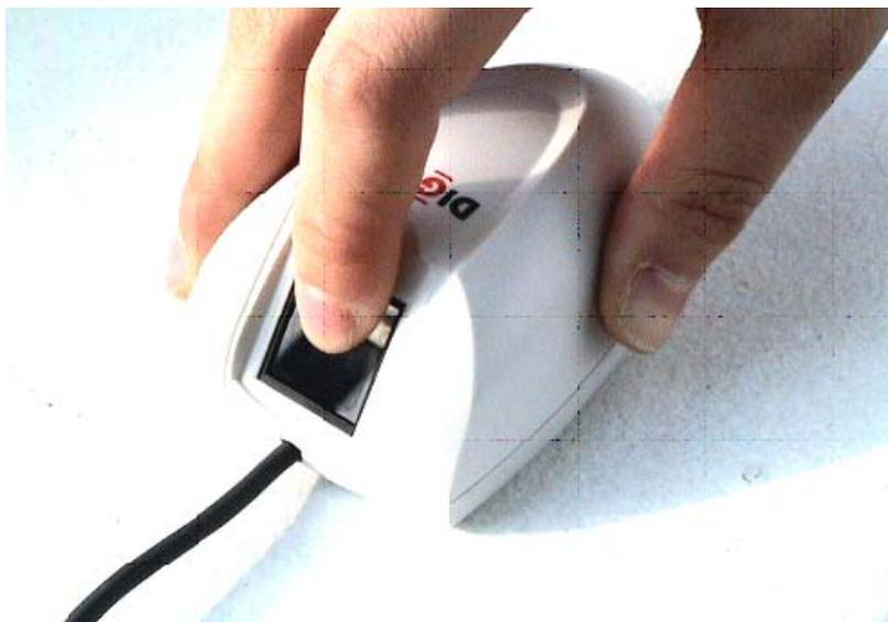
Another WRONG example of finger positioning. The core is slightly to the right of the image sensor.
